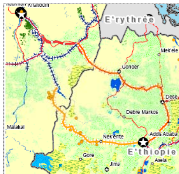
Figure 62. Railway ayout of Sennar – Addis Abeba section (850 km according to a first alternative and 1050 km according to a second variant)
